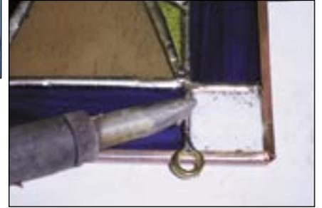
Cap the edge of the glass with copper U-channel, then solder the hangers in place.
