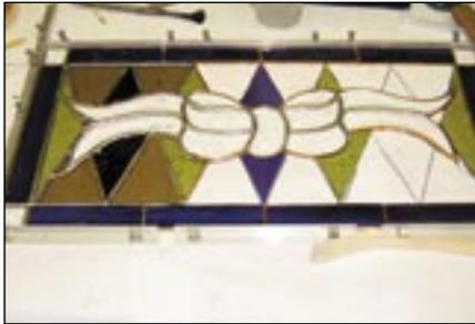
Cut, fit, grind, and foil the glass.
